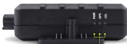
Strom-LED / GPS-LED / CEL-LED
